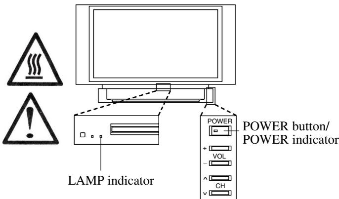
1. Switch off power to the television, wait until the power indicator stops blinking red, then unplug the power cord from the wall outlet. **Allow the television to cool for at least 1 hour.**
