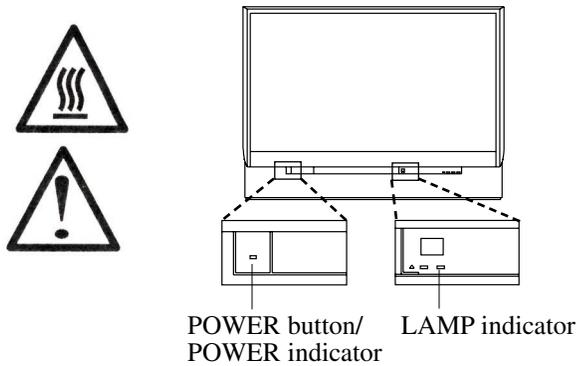
1. Switch off power to the television, wait until the power indicator stops blinking red, then unplug the power cord from the wall outlet. **Allow the television to cool for at least 1 hour.**
