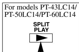
2. While pressing the VOL- button on the projection display, hold down the PIP or SPLIT button on the remote control simultaneously for more than 5 seconds.
