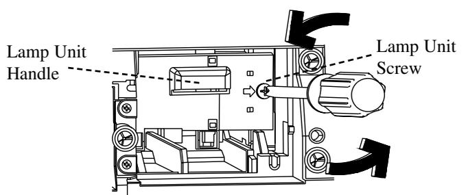
4. Using a screwdriver, loosen the lamp unit screw. Grasp the lamp unit handle and slowly pull the lamp unit from the projection display.
