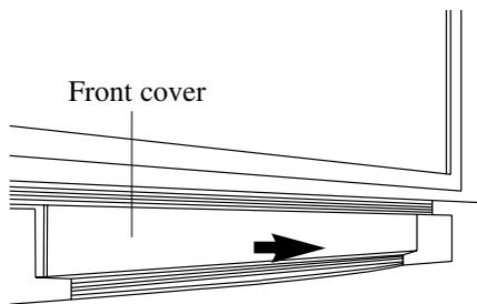
2. **Remove the front cover.** Place your fingertips under the front cover and pull it from the projection display.
