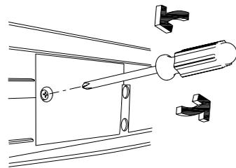
3. **Loosen the lamp cover screw.** After reading the caution and warning labels on the lamp cover, loosen the lamp cover screw using a screwdriver.
