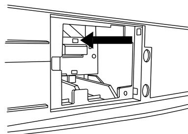
5. **Insert the new lamp unit,** paying attention to the direction of insertion. Press on the lamp unit handle, ensuring that the insertion is done correctly. Dispose of the old lamp in accordance with local environmental regulations. Tighten the lamp unit screw and the lamp cover screw using a screwdriver. Replace front cover.
