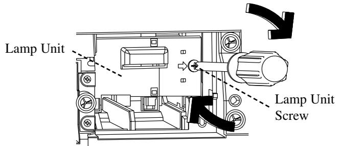
5. Insert the new lamp unit, paying attention to the direction of insertion. Press on the lamp unit handle, ensuring that the insertion is done correctly. Dispose of lamp in accordance with local environmental regulations. Tighten the lamp unit screw with using a screwdriver.
