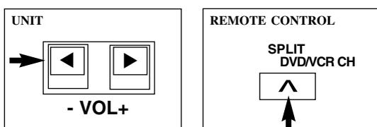
2. While pressing the VOL- button on the projection display, hold down the SPLIT button on the remote control at the same time for more than 5 seconds.
