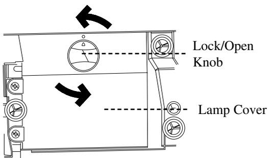
3. Turn the Lock/Open knob to the left (counterclockwise). Pull the lamp cover out and down to open it.
