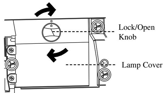
6. Close the lamp cover. Turn the Lock/Open knob to the right (clockwise).
