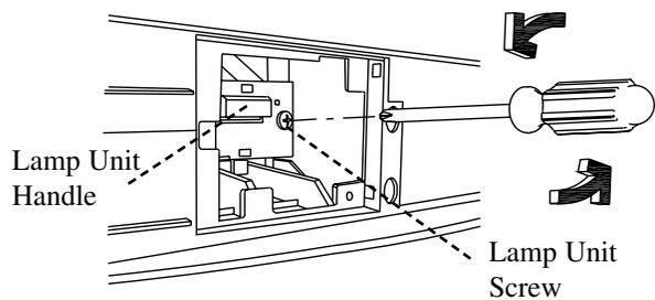
4. **Loosen the lamp unit screw.** Using a screwdriver, loosen the lamp unit screw. Grasp the lamp unit handle and slowly pull the lamp unit from the projection display.
