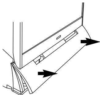
2. Grasp both sides of the front cover with your fingertips and pull it from the projection display for removal.
