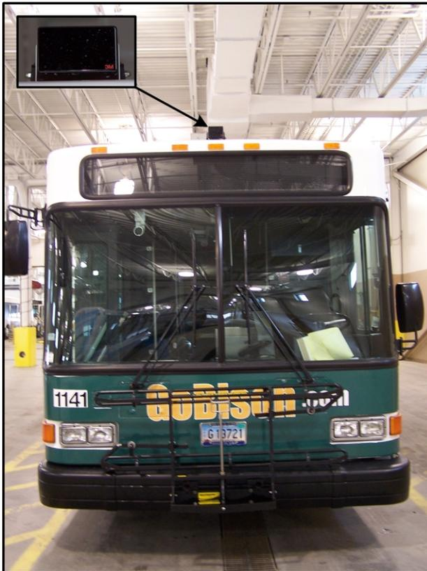
Figure 4. Bus equipped with Opticom emitter
