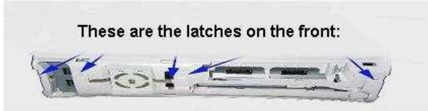
Once you have them all separated, pull off the bottom of the Xbox 360, be very gentle. Now, from the bottom of the Xbox 360 carefully flip the Xbox back over. Remove the DVD button arm assembly to keep it out of your way. You just need to gently pry it off the black plastic guide. Next, remove the top cover, watch the DVD button latch! (it is seated in the front metal casing) Disconnect the SATA connector from the motherboard and lift the DVD drive out of the case.
