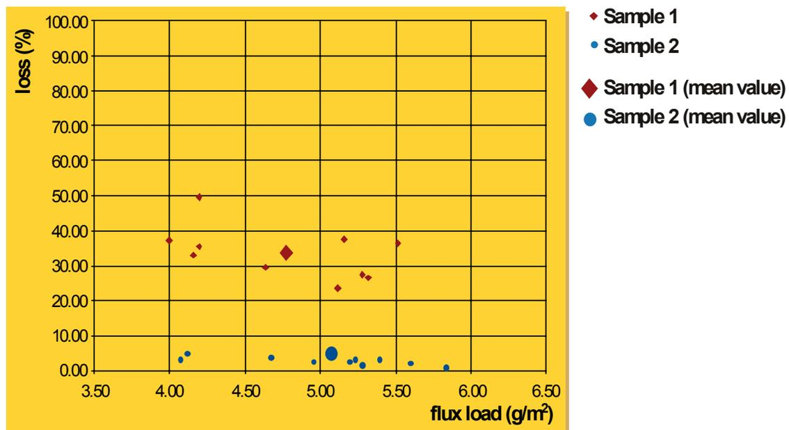
Flux powder is electrically charged in the gun. Usually, adhesion in electrostatic application is dependent on electrical forces. The flux loses the charge when it hits the grounded heat exchanger. Gravitational forces are now competing with relatively weak Van-der-Waals forces. This explains why fine particles adhere better.
