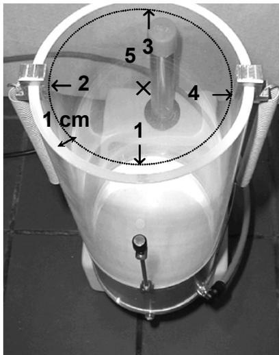
Indication of the locations for the measure of the height of the powder in both fluidized and non fluidized condition.
