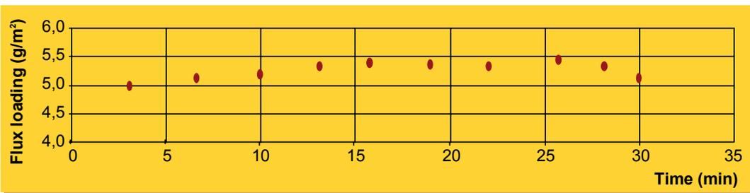
**Table 3: Flux Deposition on a Heat Exchanger (30 Minutes Test)**
