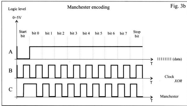
The encoding is simply an exclusive-OR function between the data and a clock frequency of twice the bit rate. This can be carried out either in software, if a microprocessor or microcontroller is generating the data to be transmitted, or using an XOR gate and perhaps a D-type to synchronise the data to the clock frequency if required.
