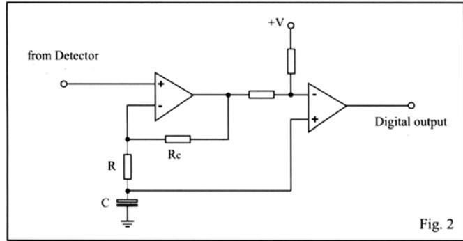
Fig. 2 Schematic diagram of Receiver (LF)
