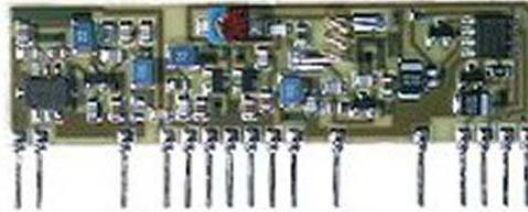
Digital data transceiver module suitable for half-duplex two-way radio transmission with fast RX-TX switching. A wide LF bandwidth allows data rates of up to 4800 baud .
