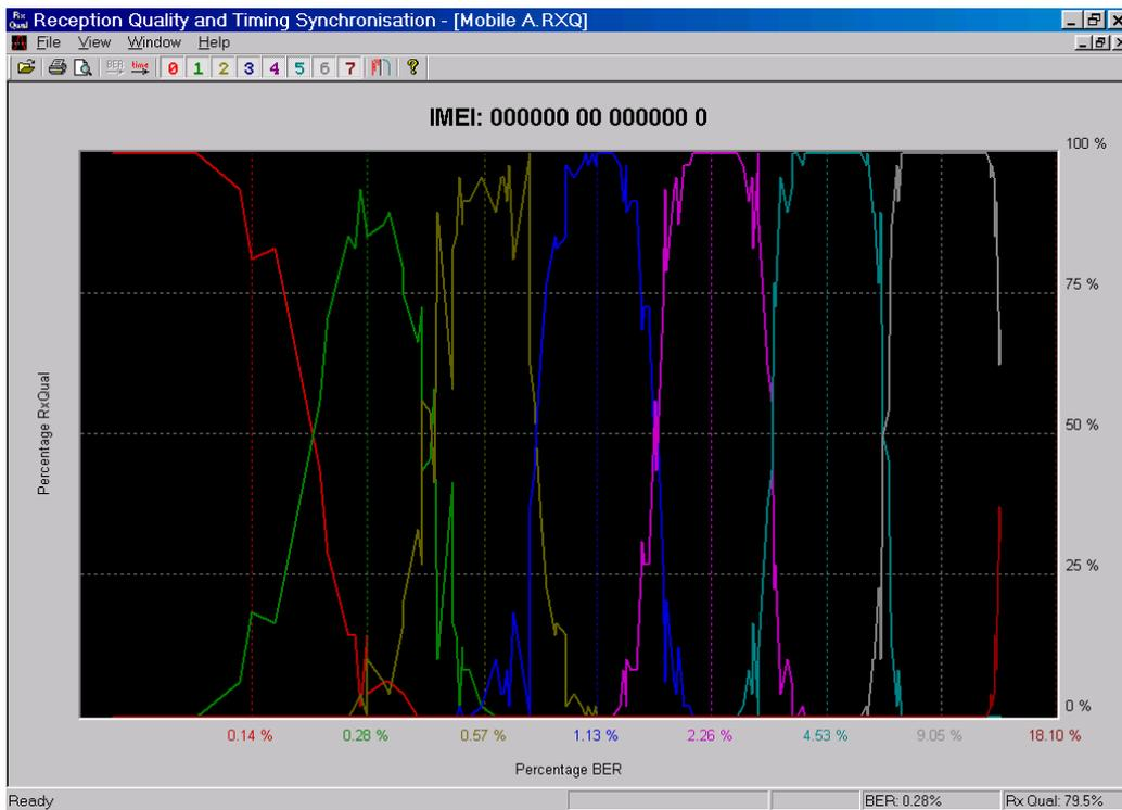
Fig. 2: RxQual vs BER in response to level change
