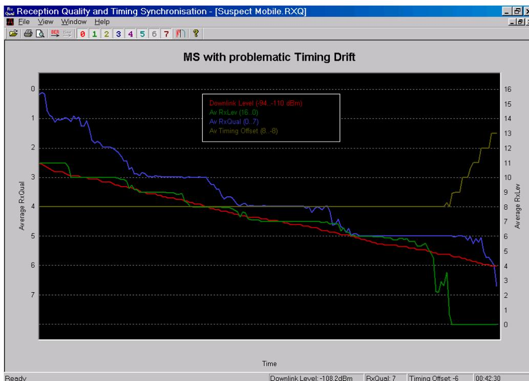
Fig. 1: RxQual, RxLev and Timing response to level change against time
