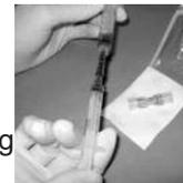
Sterile connector-double female ends for mixing between luer lock or luer slip syringes.
