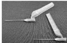
One-handed activation. No solid surface required. Simple finger stroke activation. Protective arm keeps fingers behind needle. An audible click as well as tactile feel and visual indicator confirm safety mechanism engagement. Needle remains locked inside activated cover. Fits any brand syringe. 100/box
