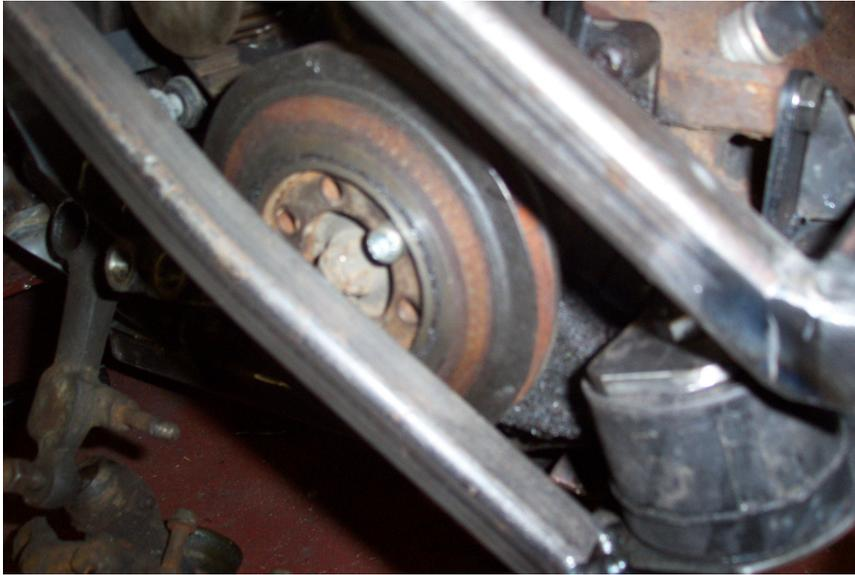
The plug head on the back of the oil filter housing needs 4mm machining off and the housing it screws into needs reducing by 7mm, ie. By sawing off ensuring the cut is square, the plug then needs refitting with a good thread sealer ie. Ptfte tape. As shown. This gives clearance to the o/s top arm pivot shaft.
