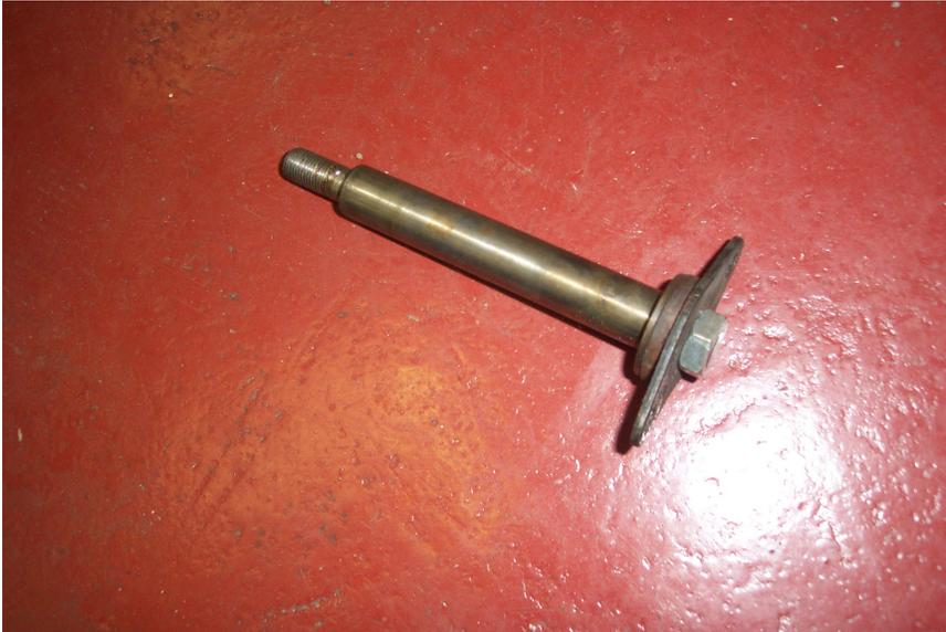
The subframe can now be lifted into position, passing the large original top bolts through the new steel washers (included). Show below
