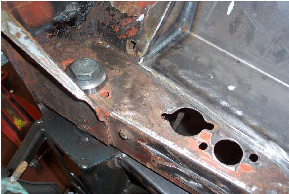
Then bolt the rear mounts to the floor.
