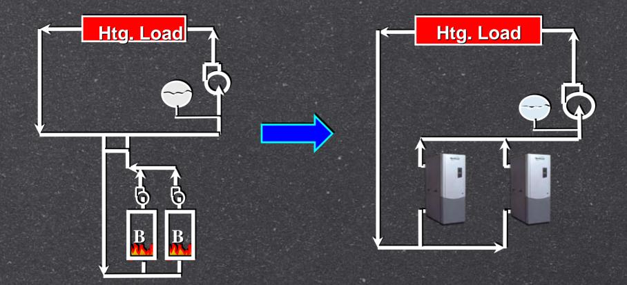
Reduce/Eliminate Material and Labor: Primary-Secondary Pump, Piping, Elect., Controls, Maintenance AND Improve System Reliability
