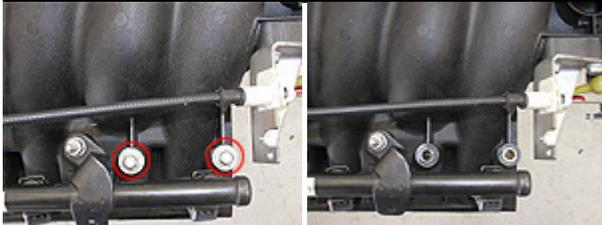
As viewed from above, locate the two intake manifold bolts as shown inside the small red circles in the picture at the far left. Remove and save these two bolts.
