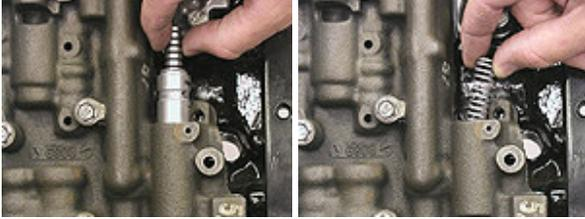
You will then need to remove the TV Plunger and the bushing. To do this, simply pull the TV plunger and bushing out. Now remove the old spring. If the TV plunger and bushing prove difficult, you can make the TV plunger act as a slide hammer by simply pushing it all the way in, release it in such a way as to cause it to "snap" back out, repeat this action as necessary until you get it removed.
