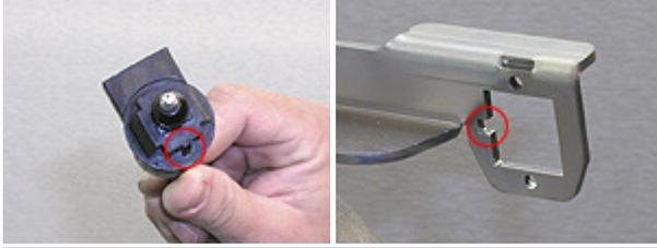
Insert the TV cable into the base plate bracket until you hear it click into position. To do this, match the index guide on the TV cable housing, with the notch in the base plate bracket (red circles in pictures at left). The TV cable will not go in any other way.
