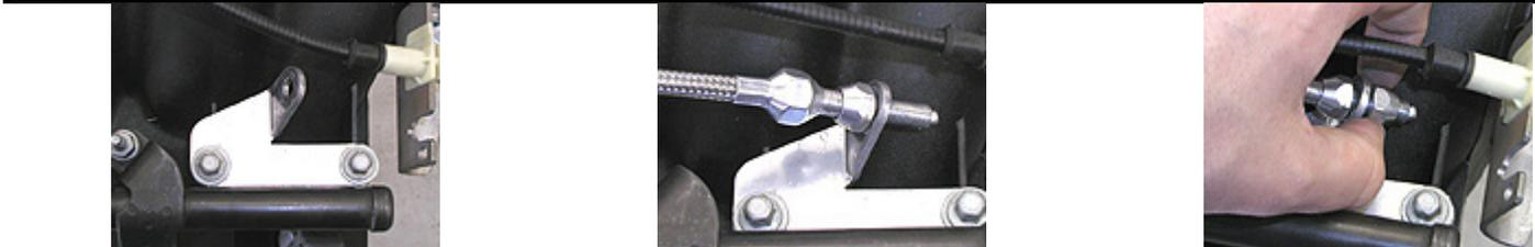
Install the new bracket pictured above onto the manifold using the original bolts you removed in step 5. Tighten to factory specifications. Install the new stainless steel cable to the transmission end first per the following link instructions then attach the cable to the intake manifold bracket as shown above.
