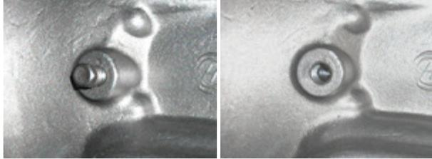
The pressure gauge must be connected to the transmission at the location shown above. This is a direct fluid passage to the transmissions internal hydraulic pump. This **installation** will be done while the engine not running. **Testing** will be done with the engine running. To hook up the gauge, locate the 1/8" plug on the "Driver Side" of the transmissions bell housing as shown in the above pictures; unscrew the plug from the transmission.
