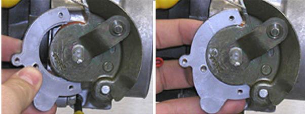
Locate the back plate/spacer plate piece in the TV Made EZ kit (far left picture). Notice that this part has a lipped section on the inside radius. Using this lip as a guide, place this adapter onto the LS-1 linkage from the back side as shown in the picture near left. This part is designed to fit snugly so a light amount of force may be needed for installation.
