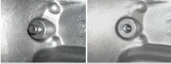
The TV cable is connected to the passenger side of Th-2004R and Th-700R4 transmissions at the locations shown in the above pictures. Same side as your dipstick. The picture at the far left shows the wire link and the TV cable to case seal. This seal must be placed into the transmission before installation, *not onto the end of the TV cable housing!* The wire link will be inserted into the hole of the connector at the transmission end of the TV cable. (See closest picture at left)
