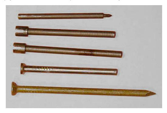
**Now the rare bits;** (Of which I have a few) HSA 269 - S5 Primary Sun Pinion \$12.00 *http://bikesmithdesign.com/SA/S5andFWsuns.jpg* The FW sun is on the axle. As one side of the dogs are ramped, it will only transmit power in one direction.
