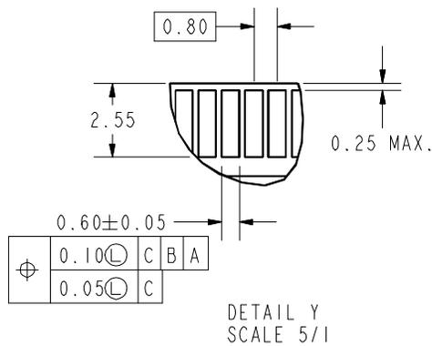
Figure 6: SO-DIMM Mechanical Drawing (4 of 5)
