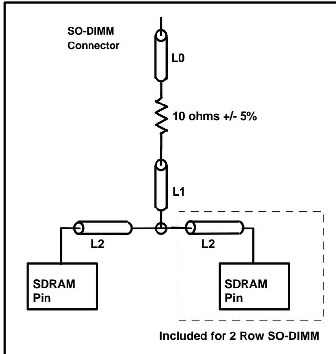
Note: The L1 trace segment may contain up to 2 additional vias which are not shown in the diagram.
