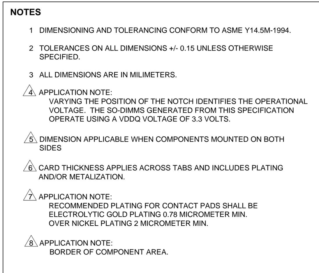
Figure 7: SO-DIMM Mechanical Drawing (5 of 5)
