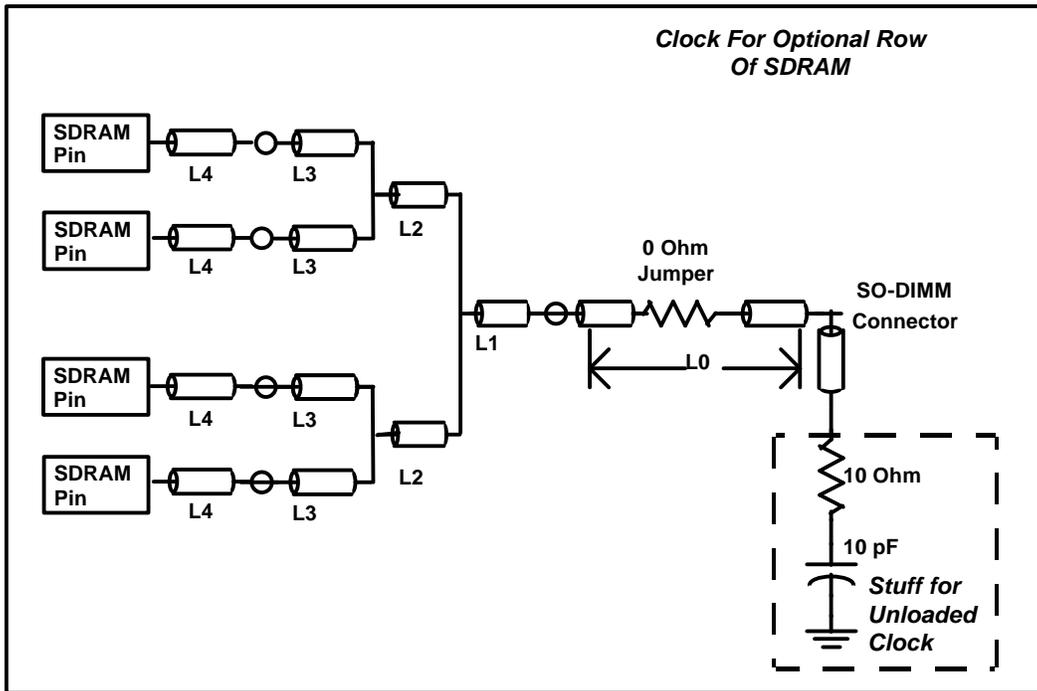
Note: Either the L2 or the L3 trace segment may contain one additional via which is not shown in the diagram.
