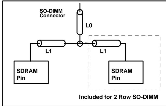
Note: The L0 trace segment may contain 1 additional via which is not shown in the diagram.
