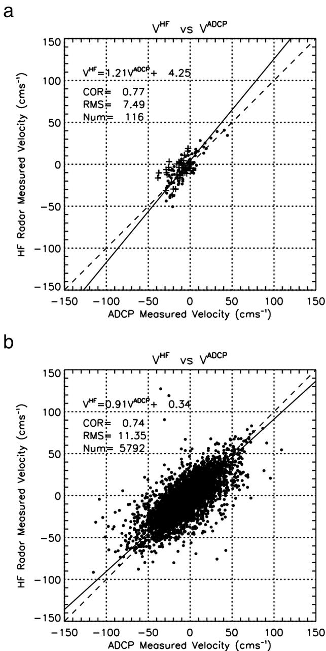
**Figure 5.** Scatterplots of ADCP measured velocity (horizontal axis) and HF radar measured velocity (vertical axis). (a) ADCP (RD Inc., 150 kHz) towed by T/V *Kakuyo-Maru* (circle) and ADCP (RD Inc., 600 kHz) mounted on R/B *Danryu* (plus). Data at 13 m depth were used. (b) ADCP (Furuno Inc., 150 kHz) mounted on T/V *Kakuyo-Maru*, patrol ships of 7th RCGH, and research ships of FFMTRC. Shallowest data at 5~9 m depth were used. Solid line is the regression line obtained with PCA.
