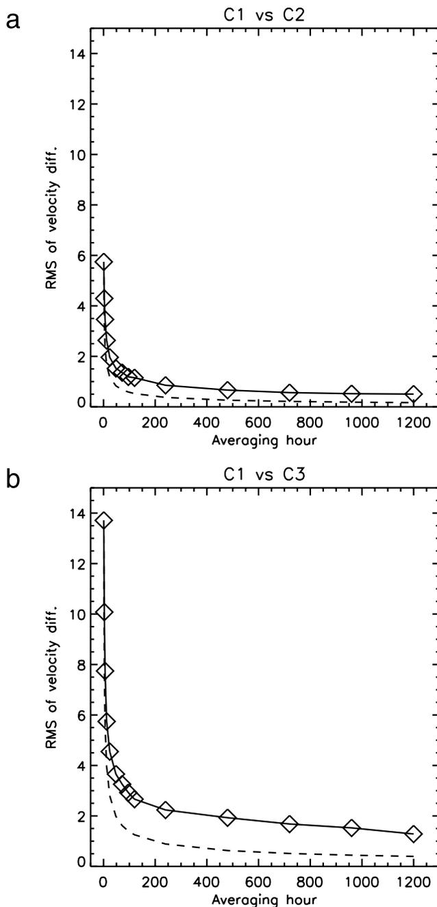
**Figure 7.** RMS obtained from facing radar comparisons as a function of ensemble number of averaging. (a) C1–C2 comparison. (b) C1–C3 comparison. Dashed line represents inverse of square root of ensemble number.
