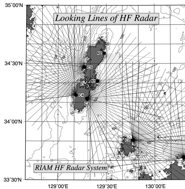
**Figure 3.** Location of HF radar sites (CODAR, C1~C5; NJRC, N1 and N2). Looking lines and range coverage of each radar are drawn by lines.
