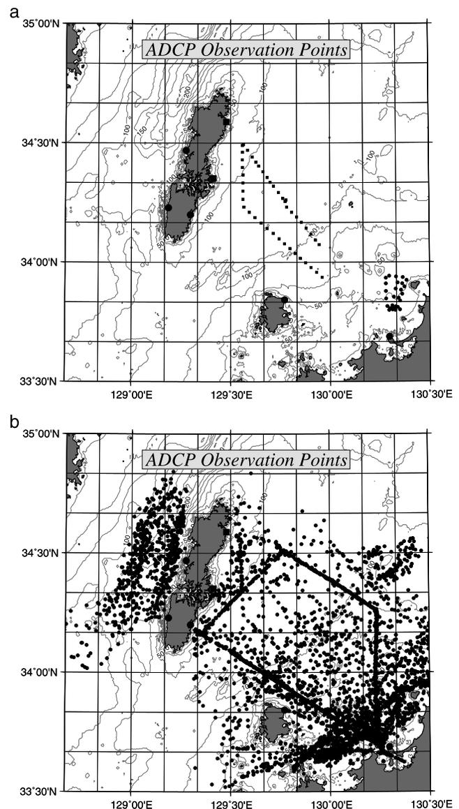
**Figure 4.** Locations of ADCP measurements. (a) ADCP (RD Inc., 150 kHz) towed by T/V *Kakuyo-Maru* (square) and ADCP (RD Inc., 600 kHz) mounted on R/B *Danryu* (circle). (b) ADCP (Furuno Inc., 150 kHz) mounted on T/V *Kakuyo-Maru*, patrol ships of 7th RCGH, and research ships of FFMTRC.
