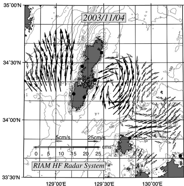
**Figure 2.** Example of anticlockwise eddy observed in the eastern channel of the Tsushima Strait.
