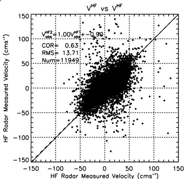
**Figure 6.** Scatterplots of radial velocities measured by two facing HF radars. (a) C1–C2 comparison. (b) C1–C3 comparison. Solid line is the regression line obtained with PCA.
