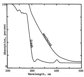
Figure 3 Ultraviolet spectra of fresh and of weathered Incralac.
