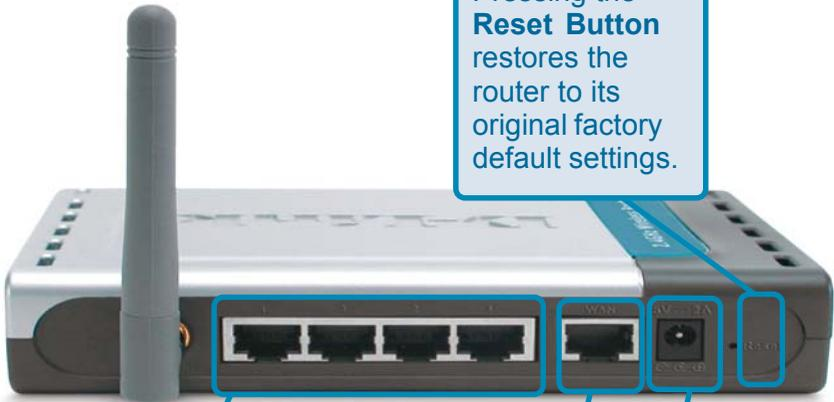
**Auto MDI/MDIX LAN ports** automatically sense the cable type when connecting to Ethernet-enabled computers.
