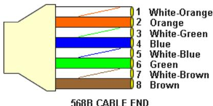
All you need to remember to properly configure the cables is the pinout order of the two cable ends and the following rules:
