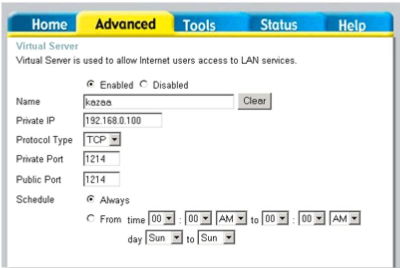
The screenshot shows the 'Virtual Server' configuration page in a router's web interface. The page has a navigation bar with tabs for 'Home', 'Advanced' (which is selected), 'Tools', 'Status', and 'Help'. Below the navigation bar, the page title is 'Virtual Server' and a description reads 'Virtual Server is used to allow Internet users access to LAN services.' The configuration options are as follows:
