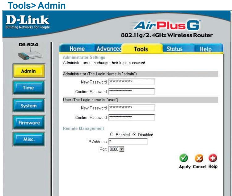
At this page, the DI-524 administrator can change the system password. There are two accounts that can access the Broadband Router's Web-Management interface. They are admin and user. Admin has read/write access while user has read-only access. User can only view the settings but cannot make any changes.
