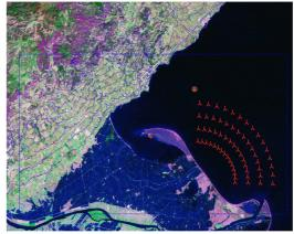
bands, each sensible to the different parts of the reflected solar energy. It is possible to convert individual bands into either true colour pictures or artificial (false) colour pictures. The option of using artificial colour pictures are widely used within the field of remote sensing, i.e. when studying changes in global vegetation, pollution etc.
