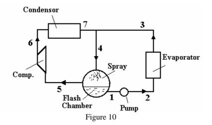
Further modifications may be made by compressing the vapour in two stages and mixing the vapour from the flash chamber at the inter-stage point. The output of the evaporator then goes to the input of the low pressure stage as shown in fig.10
