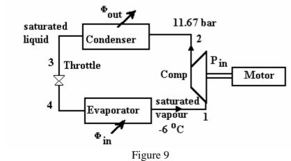
$h_1 = h_f \text{ at } -6^{\circ}C = 1437.6 \text{ kJ/kg}$   $h_3 = h_4 = h_f @ 11.67 \text{ bar} = 323.1 \text{ kJ/kg}$  $s_1 = s_f \text{ at } -6^{\circ}C = 5.419 \text{ kJ/kg K}$  Ideally  $s_2 = s_1 = 5.419 \text{ kJ/kg K}$
