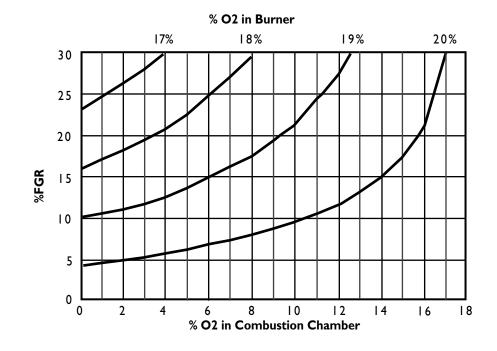
The other thing to consider is the temperature of the air/flue gas mixture in the combustion air blower. Let's say the manufacturer says the blower shouldn't be exposed to more than 250°F, and the flue gas temperature is 700°F. The blend temperature chart (Figure 3) shows that a mixture containing 20% of 700°F flue gases, the rest 80°F air, will have a temperature of 210°F, which is below the limit for the blower, so you have the makings of a good FGR installation
