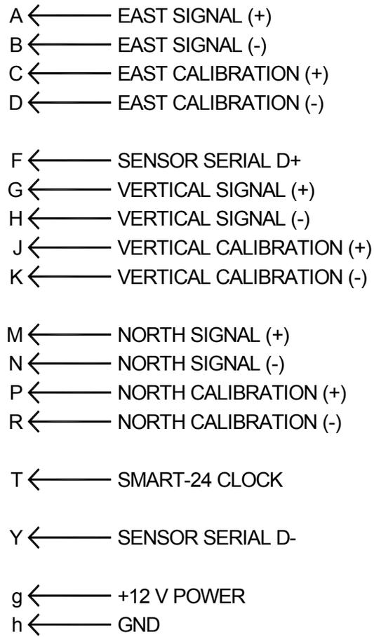
Figure 2.1 Circular Output Connector Pin Definition of Triaxial Accelerometer
