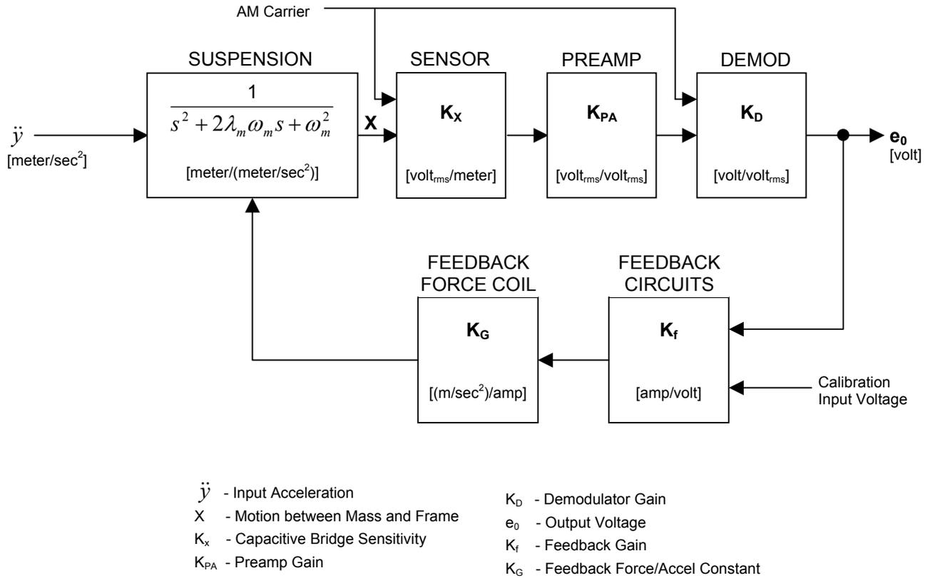
Figure 3.1 FBA Block Diagram
