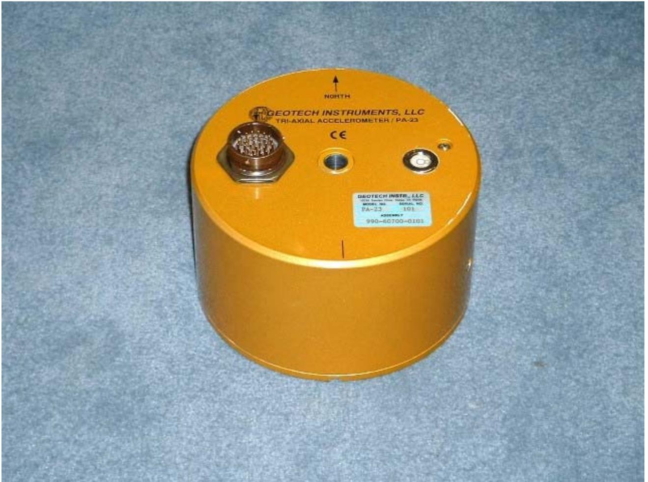
Figure 2.2 Triaxial Accelerometer, Model PA-23
