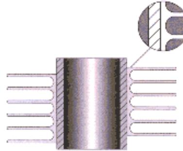
Detail for the tube and fin section in the heat exchanger
