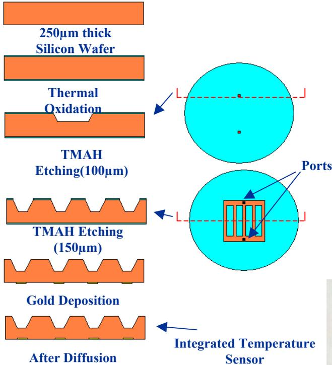
Established fabrication process for microchannels
