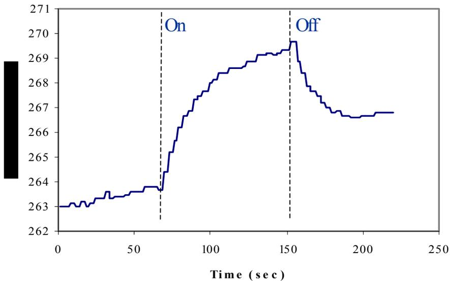
Change in temperature (~ 6K) with time at initial temperature 263.8K
