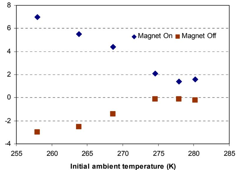
Change in temperature at various initial ambient temperatures
