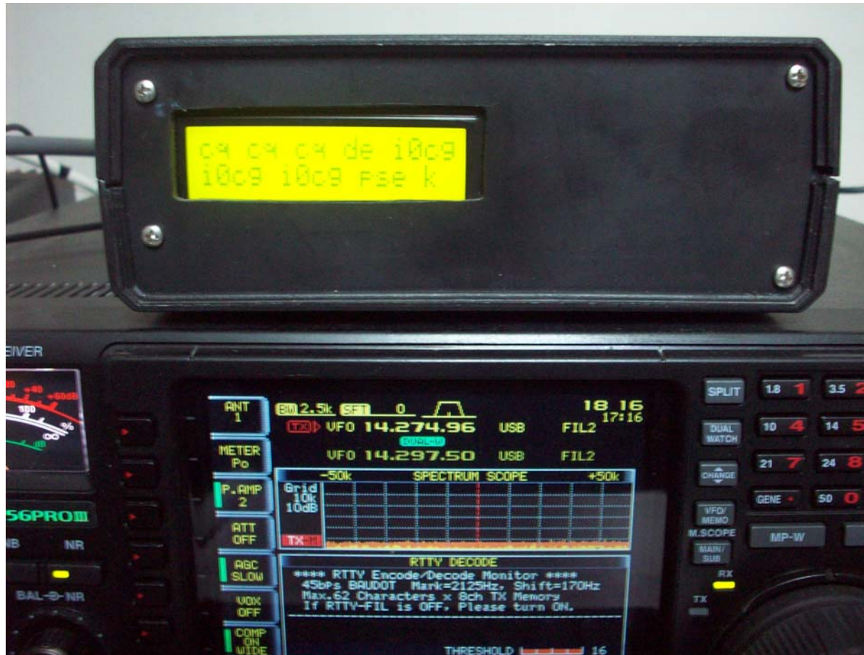
RTTY interface inside a prototype box in use with my IC-756proIII
