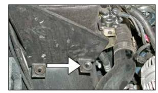
7. Remove the air box mounting grommet as shown.
