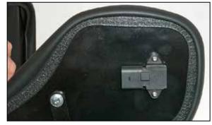
12. Install the temperature sensor onto the heat shield with the provided hardware as shown.
