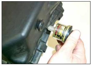
21. On vehicles that are equipped with a filter minder.
