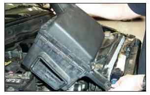
6. Remove the complete air box assembly from the vehicle as shown.
