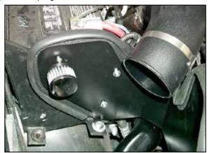
24. Install the K&N<sup>®</sup> air filter onto the air
