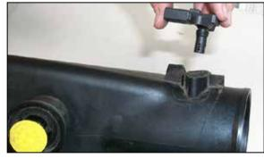
11. Remove the temperature sensor from the air box lid using an 9/32 socket.
