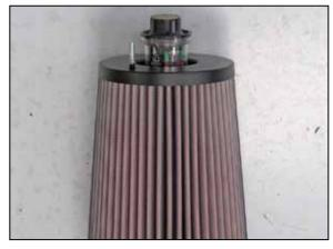
23. On vehicles equipped with a filter minder, install the factory grommet and filter minder into the K&N air filter as shown. On vehicles that are not equipped with the facory filter minder, install the provided plug into the filter
