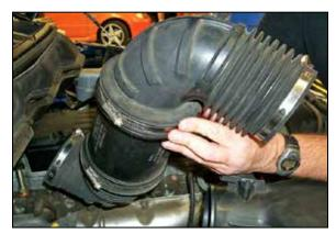
4. Remove the intake tube from the vehicle as shown.
