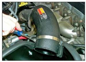
22. Install the intake tube onto the turbo inlet, then align with the saddle bracket. Attach the saddle bracket to the intake tube with the provided hose clamp, adjust the bracket to achieve the appropriate clearance for the intake tube before tightening.
