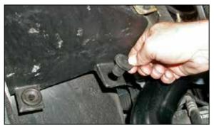
14. Install the nut insert onto the air box mounting tab as shown.
