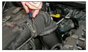
3. Loosen the hose clamps at the turbo inlet and the air box outlet as shown.
