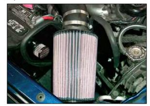
25. Install the K&N $^{\ensuremath{\mathbb{R}}}$  air filter onto the intake tube as shown.
