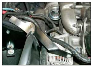
19. Install the saddle bracket assembly onto the alternator with the bolt that was removed in the previous step.
