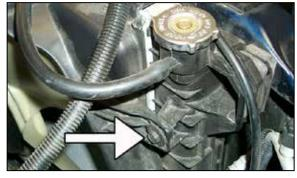
13. Remove the bolt that retains the fan shroud to the radiator.
