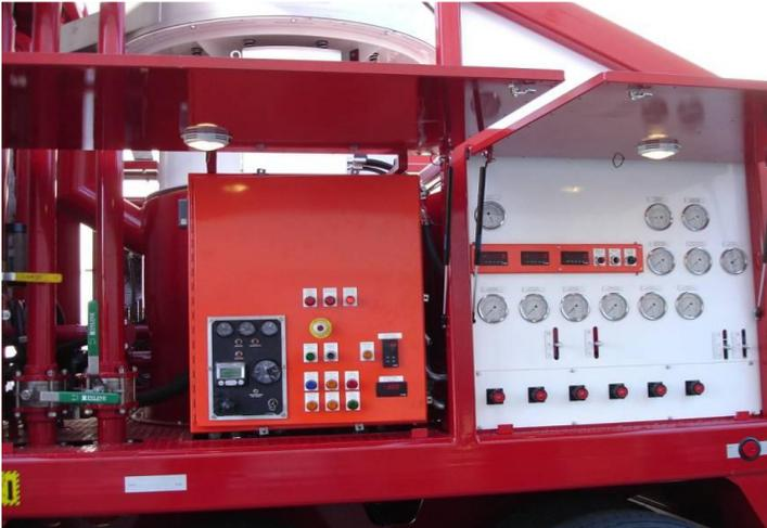
System has latch doors to protect control panels during transportation, and bad weather during system operation are equipped with head lights for night operations.
