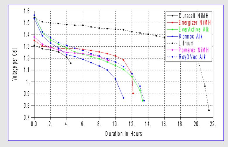
The following table is the recorded data used presented in the graph above. The orange highlighted data below is when the GPS unit shut itself off as indicated by a rise of voltage on the DVM. The unit emits a low level alarm before this voltage, but gives you very little reserve time, from none to several minutes.
