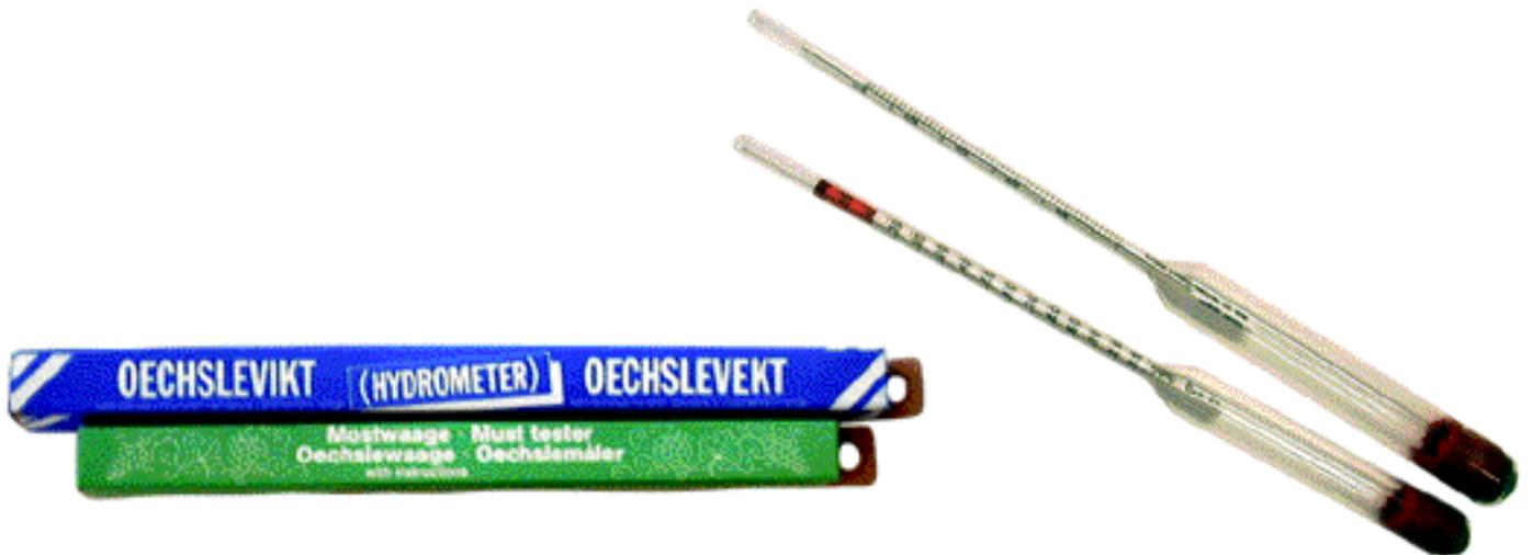
This hydrometer measures wine and other fermentations. It is of laboratory quality, and is not sold in home brew shops. While a laboratory quality hydrometer is more expensive, it gives a very accurate reading. Made by Widder, Germany.
