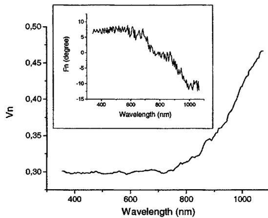
FIG. 4. PPE normalized voltage  $V_n$  spectrum of the  $65 \mu\text{m}$  EP melanin film under illumination with a white-light/monochromator system. The inset is the corresponding PPE normalized phase  $F_n$  spectrum.
