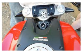
**1.** Dismount completely the handlebar mount and mount part 139/1, unscrew nuts M6 near the ignition box and remove the plastic cover.
