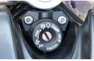
2. On the tank to the ignition box mount part 139/2 and secure with original nuts M6 (3). Mount the shock absorber to part 139/1, secure with screws M6x20. Gradually mount parts 139\_2,139\_4 and handlebars. Secure everything with screws M8x45.
