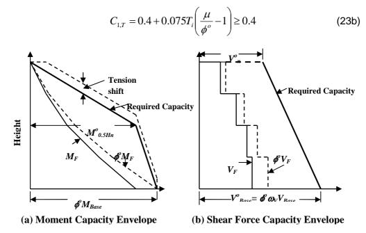
Fig. 8 Simplified Capacity Design Envelopes for Cantilever Walls
