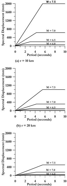
**Fig.10** Influence of Magnitude and Distance on 5% Damped Displacement Spectra for Firm Ground Using Eqs.(24) and (25) [after Faccioli et al (2005)]
