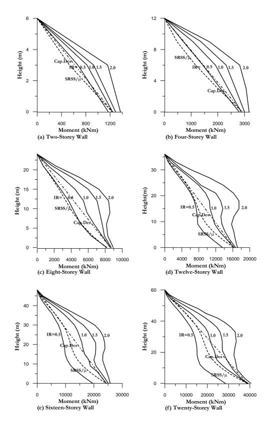
**Fig.5** Comparison of Capacity Design Moment Envelopes with Results of Time-History Analyses for Different Seismic Intensity Ratios
