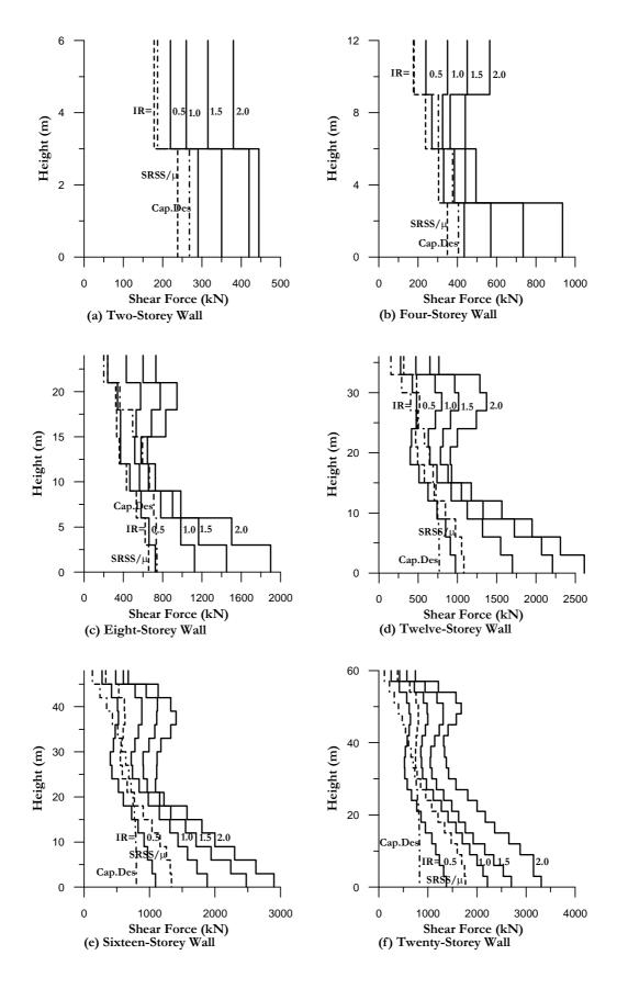
**Fig.6** Comparison of Capacity Design Shear Force Envelopes with Results of Time-History Analyses for Different Seismic Intensity Ratios
