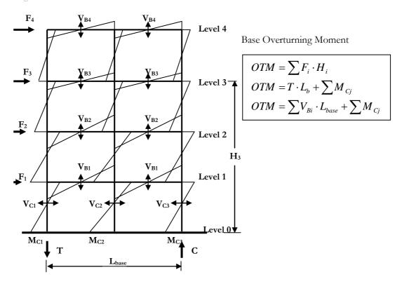
Fig.4 Seismic Moments from DDBD Lateral Forces
