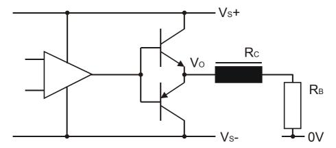
The maximum voltage, VO, will be the output swing of the op-amp less the base-emitter voltage drop of the output transistor. A conservative figure for this voltage, Vo, is (Vs -3), that is, 3 volts less than the supply voltage. This would allow a swing of  $\pm 12V$  for a  $\pm 15V$  supply.
