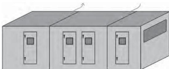
For every 1% of air leakage at the AHU, 1% more air must be conditioned, and 1% more energy is consumed.
