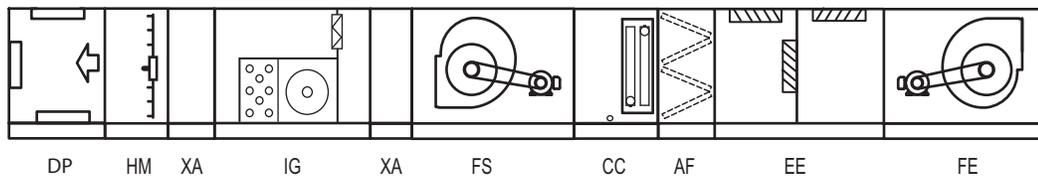
**Configuration 5 – Cooling-only lab design with HEPA filtration**
