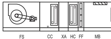
**Configuration 4 – Exhaust air flexibility with gas-heat and humidification**
