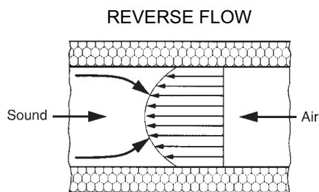
Under REVERSE FLOW conditions, sound is refracted away from the walls and toward the center of the duct-silencer.
