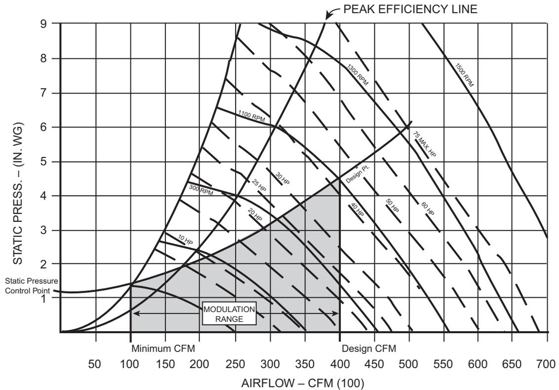
FIG. 4 – FAN CURVE AT VARIOUS RPMs
