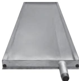
Poorly designed drain pans are often breeding grounds for mold and poor IAQ. ASHRAE 62-2001, section 5.11.1 states that drain pans "...shall be sloped at least 1/8" per foot from the horizontal toward the drain outlet whether the fan is in the on or off position." Section 5.11.2
