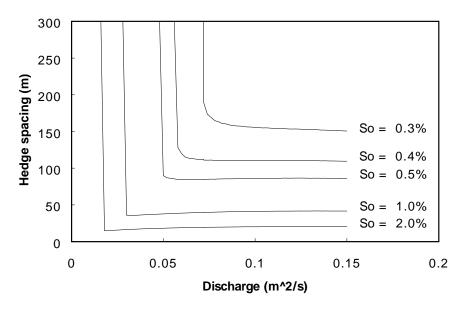
**Figure 6**: Effect of land surface slope,  $S_o$  on hedge spacing for a  $V_{max}$  of 0.5 m/s and Manning *n* of 0.03
