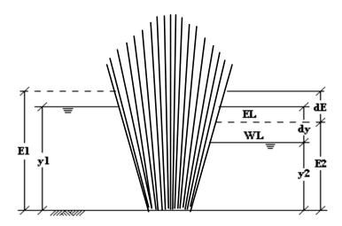
**Figure 1**: System of flow through a vetiver grass hedge and definition of terms in the discharge-depth equation
