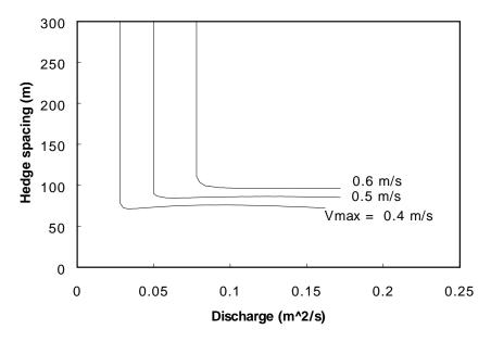
Figure 7: Effect of maximum permissible velocity on hedge spacing for a slope of 0.5% and Manning *n* of 0.03
