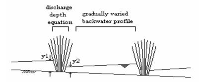
Figure 5: The physical model of flow over bare fallow and through vetiver hedges.
