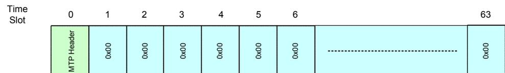
No Time Slot allocated to a VC Payload
