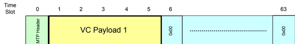
Time Slots 1-5 allocated to VC Payload 1
