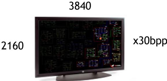
*DP v1.2 enables High Color Range Quad Full HD delivered over standard DisplayPort connector...*
