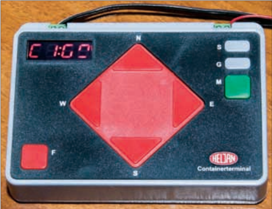
The crane ships with a pre-wired control box that allows the user to interface with the crane. The NSEW controls the back and forth movement of the gantry and the sideways motion of the crane. The S&G buttons activate the spotlight and Gantry LEDS. The M button activates the electromagnet used to lift the containers. The F is an option button that combines with other buttons to activate the hoist, etc.
