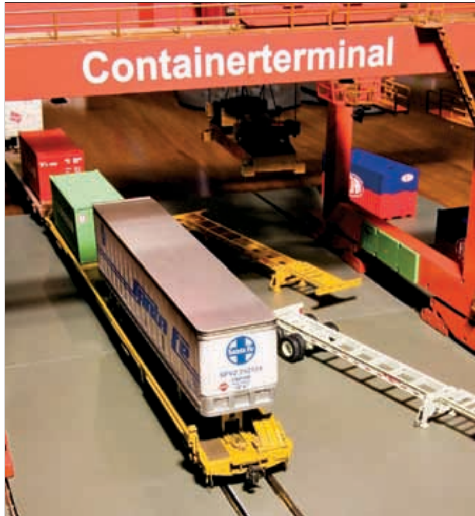
A cut of cars is spotted beneath the crane in preparation for an off-load of the containers. Although the Heljan Crane is only set up to work with 20-foot containers, metal strips can be placed inside of larger containers and inside of piggyback trailers allowing them to be moved as well. Prototypical exactness suffers when moving larger containers and piggyback trailers because the lift crane that contains the electromagnet is fixed at 20 feet. Piggyback trailers require bottom or sill lifting, and overhead lift equipment is always fitted with retractable arms that reach under the trailer to lift it. Remember that up to 5 tracks can be cut into the base, potentially creating a very busy facility.
