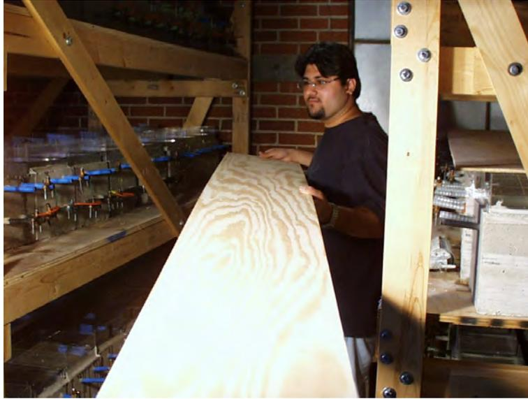
**Figure 2.22: Student Placing Plywood Sheet over Macrocell-Filled Dikes to Minimize Evaporation**
