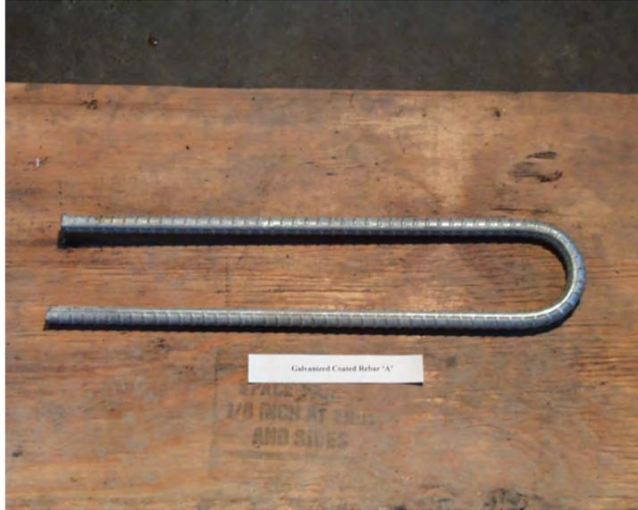
**Figure 2.7: Galvanized-Coated Reinforcement Bar A**
