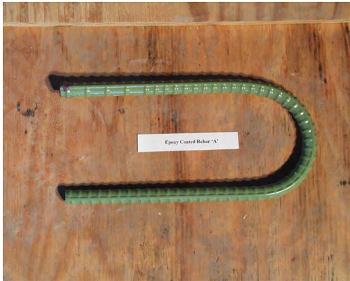
**Figure 2.2: Epoxy-Coated Reinforcement Bar A**
