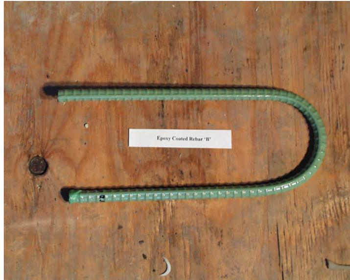
**Figure 2.3: Epoxy-Coated Reinforcement Bar B**
