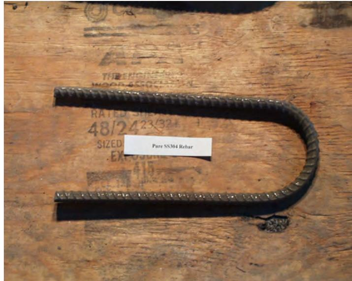
**Figure 2.9: Pure Stainless Steel 304 Reinforcement Bar**
