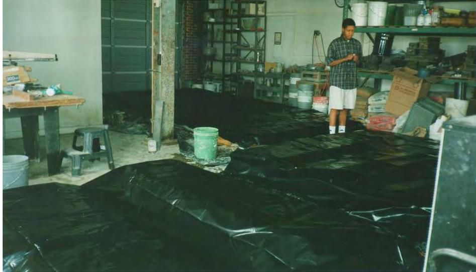
**Figure 2.16: Curing of Macrocell Specimens**
