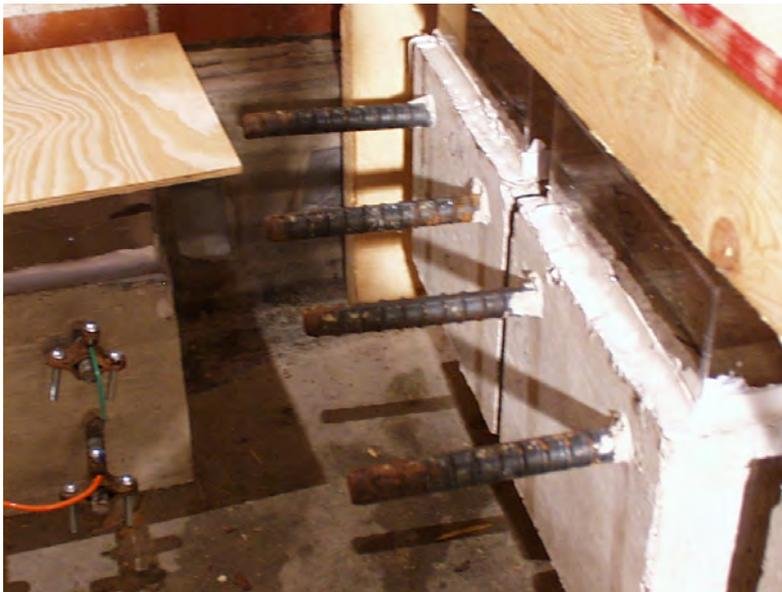
**Figure 2.23: Macrocells with One Bent Black Rebar as Top-Reinforcing Layer and None in the Bottom-Reinforcing Layer**
