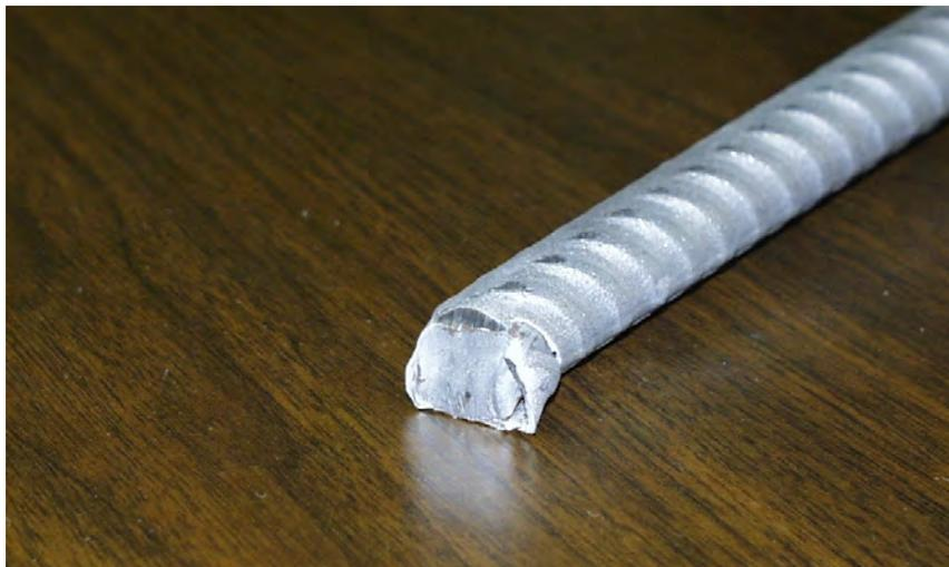
**Figure 2.12: Separation of Stainless Steel Cladding from Shearing**
