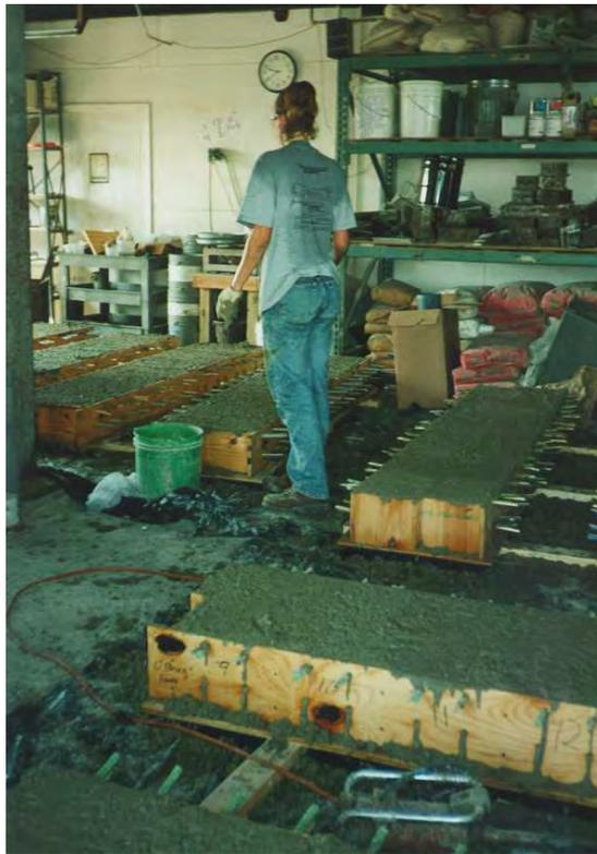
**Figure 2.15: Macrocell Concrete Placement**
