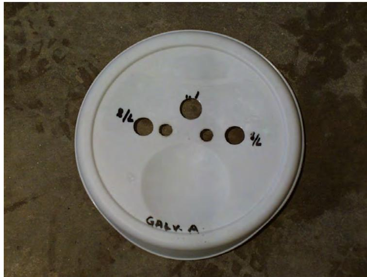
**Figure 3.5: Lid of Polarization Resistance Test Cell with Holes to Accommodate the Rebar, the Reference Electrode and the Lugin Probe**
