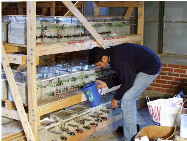
**Figure 2.21: Researcher Pouring 3.5% NaCl Solution in Dikes at Beginning of “Wetting Cycle”**
