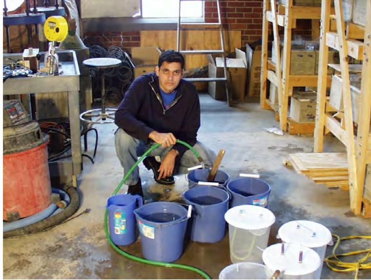
**Figure 2.20: Researcher Making 3.5% NaCl Solution at the Beginning of the “Wetting Cycle”**
