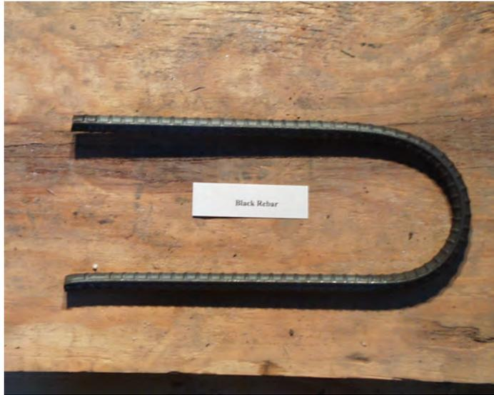
**Figure 2.1: Black Steel Reinforcement Bar**
