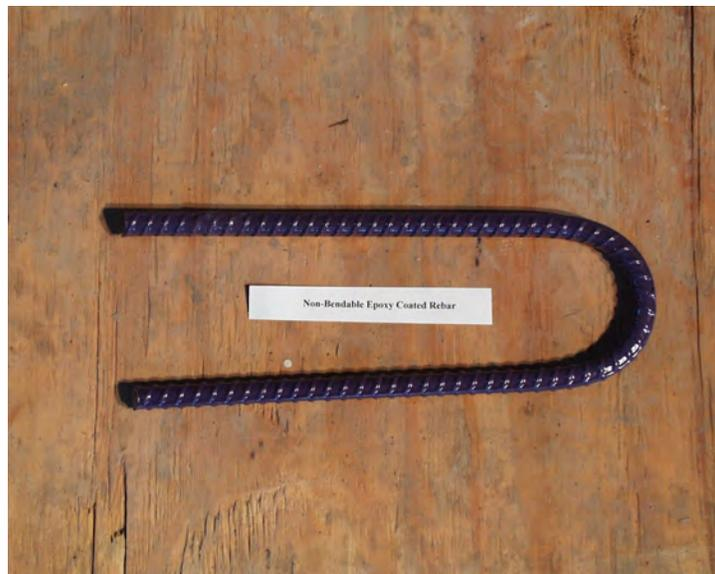
**Figure 2.4: Nonbendable Epoxy-Coated Reinforcement Bar**
