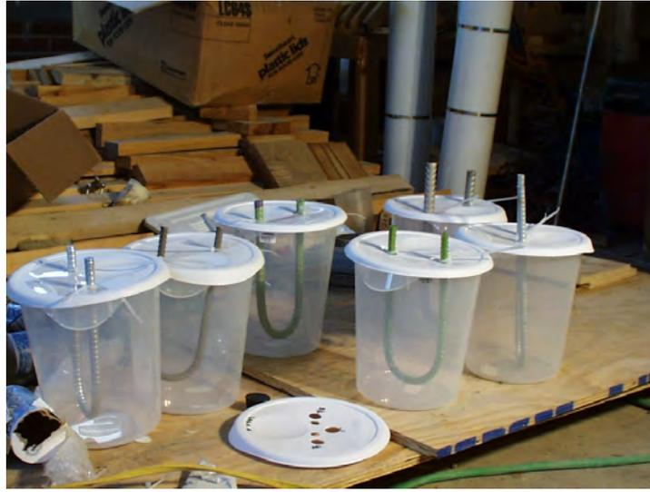
**Figure 3.3: Polarization Resistance Test Cells without Connections**
