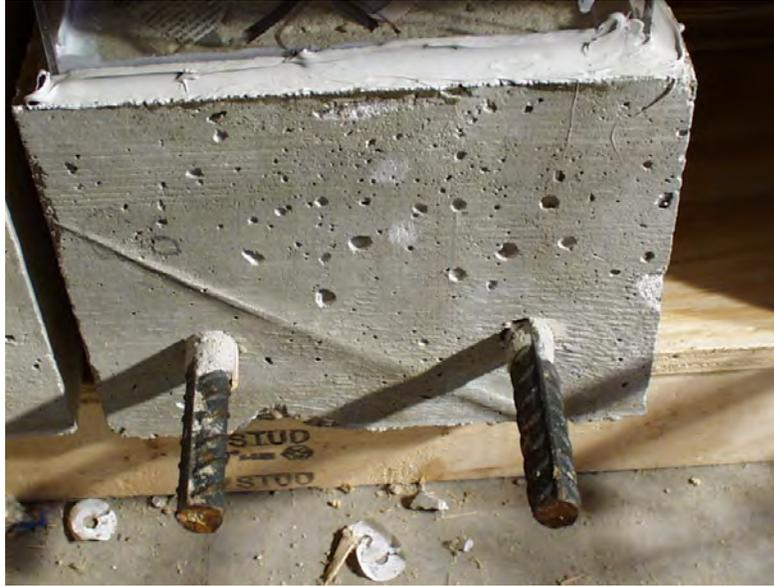
**Figure 2.24: Macrocells with Two Straight Black Rebars as Bottom-Reinforcing Layer and None in the Top-Reinforcing Layer**
