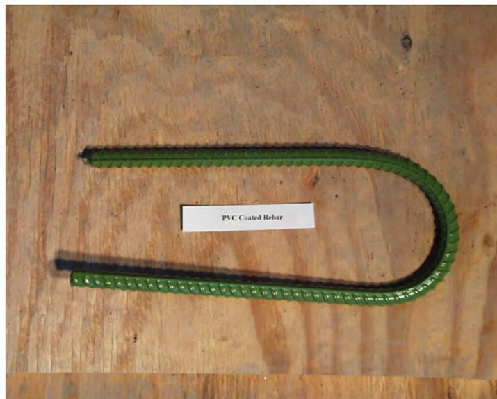
**Figure 2.6: PVC-Coated Reinforcement Bar**
