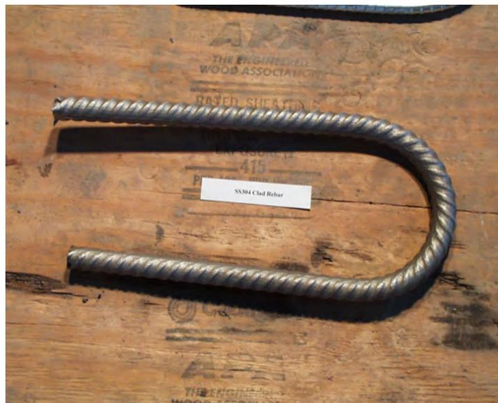
**Figure 2.10: Stainless Steel 304 Clad Reinforcement Bar**
