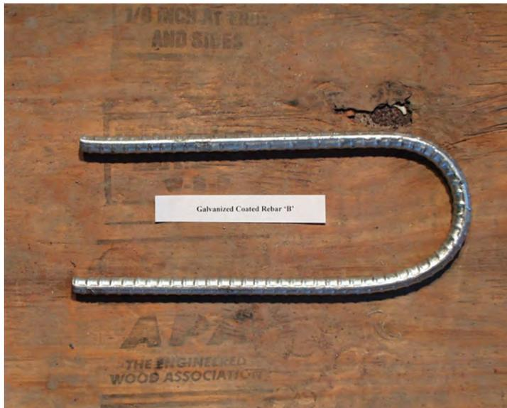
**Figure 2.8: Galvanized-Coated Reinforcement Bar B**
