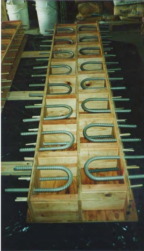
**Figure 2.14: Typical Formwork for Macrocells with #6 Bars**
