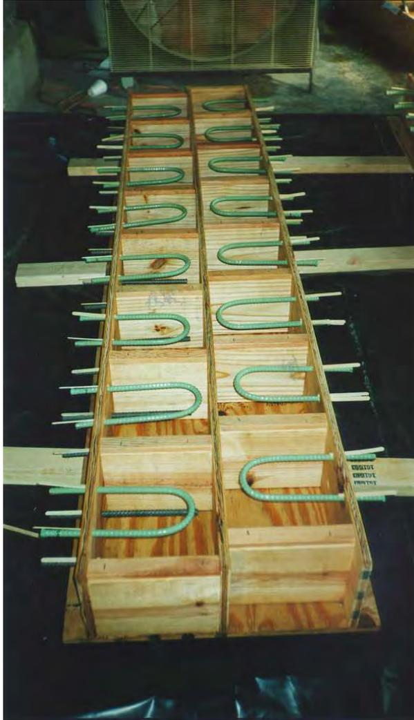
**Figure 2.13: Typical Formwork for Macrocells with #4 Bars**
