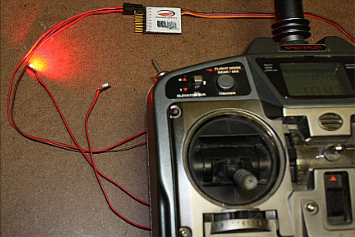
A DELight connected in parallel to a servo channel will change programs based on that servo input. This is handy if you want to make turn signals or the like.
